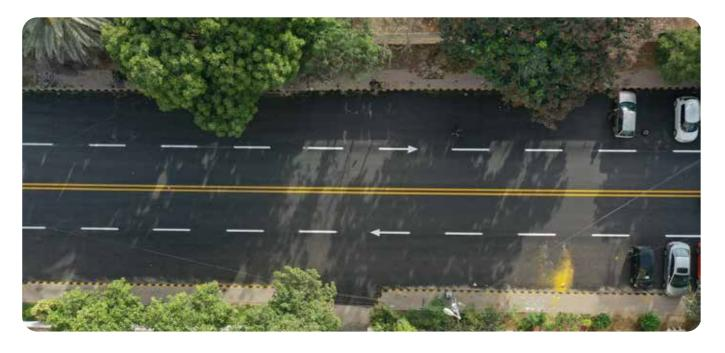
In Karachi, where Shell House is located Shell Pakistan constructed a plastic infused road surface. The road is 730 feet long and 60 feet wide and the surface contains recycled material from discarded Shell lubricant bottles. This is a purpose-built solution which is a benefit for Shell, neighboring residents, schools and the church community.
